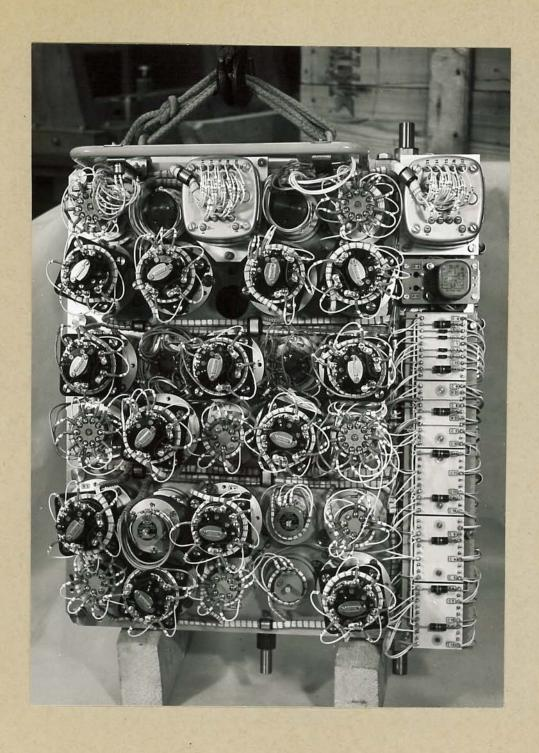
PAE IN TARGET-COMPONENTS CALCULATOR SERVO CHASSIS
