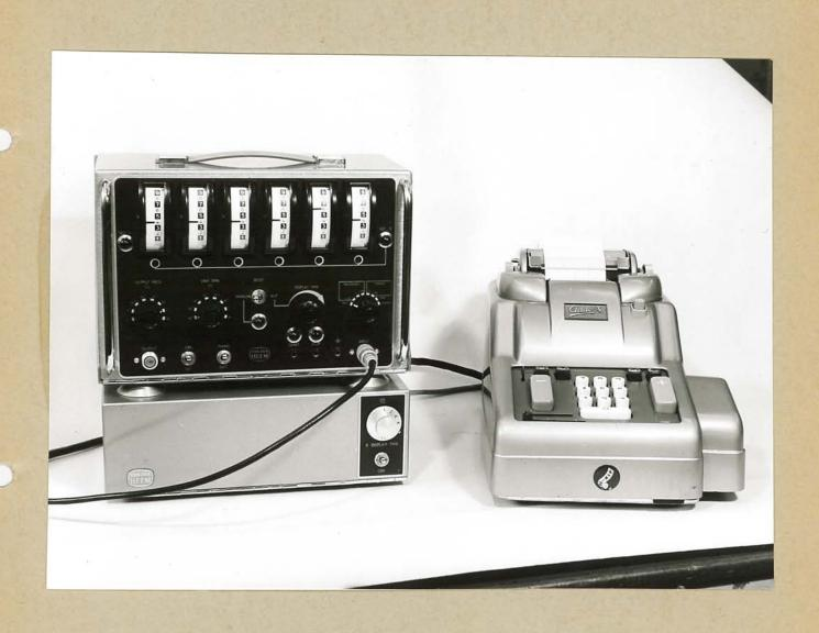
FULLY TRANSISTORIZED COUNTER WITH PRINT-OUT CONVERTER AND PRINTER
